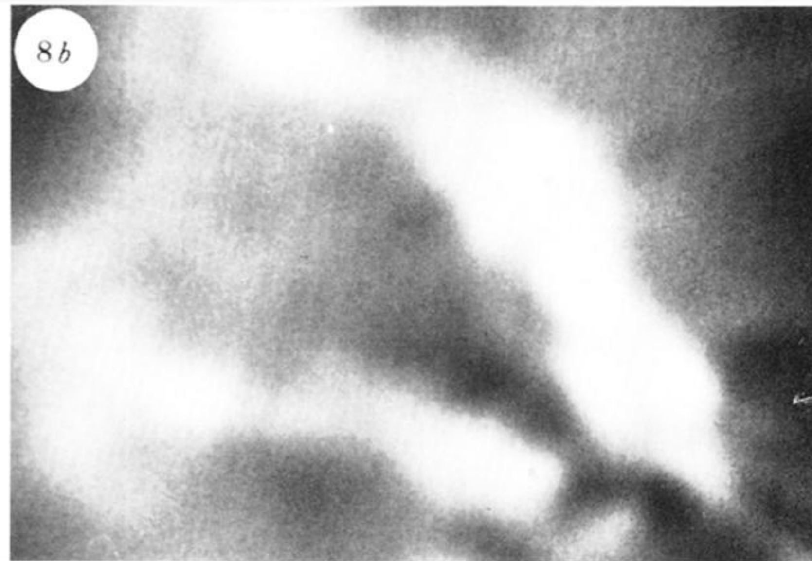
FIGURE 8. (a) SE image of a crack in an Fe–Ni–C alloy. (b) SEAM image reveals subsurface crack extending beyond visible crack tip, and also a second, completely subsurface crack.
