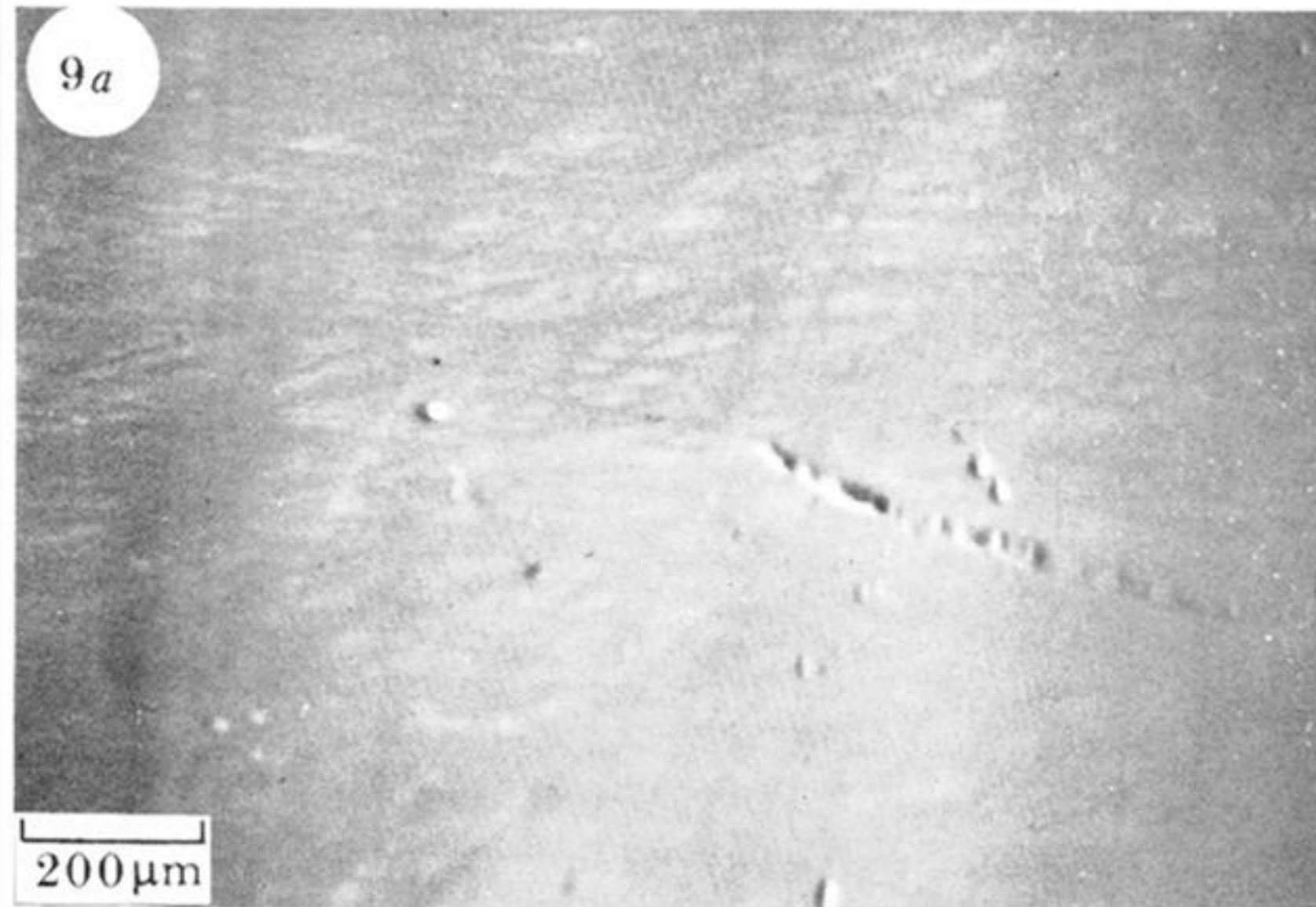
FIGURE 9. (a) SE image of a crack in polystyrene and (b) SEAM image showing craze extending beyond the crack tip. The specimen was Cu-coated and imaged at 20 keV to avoid degradation.
