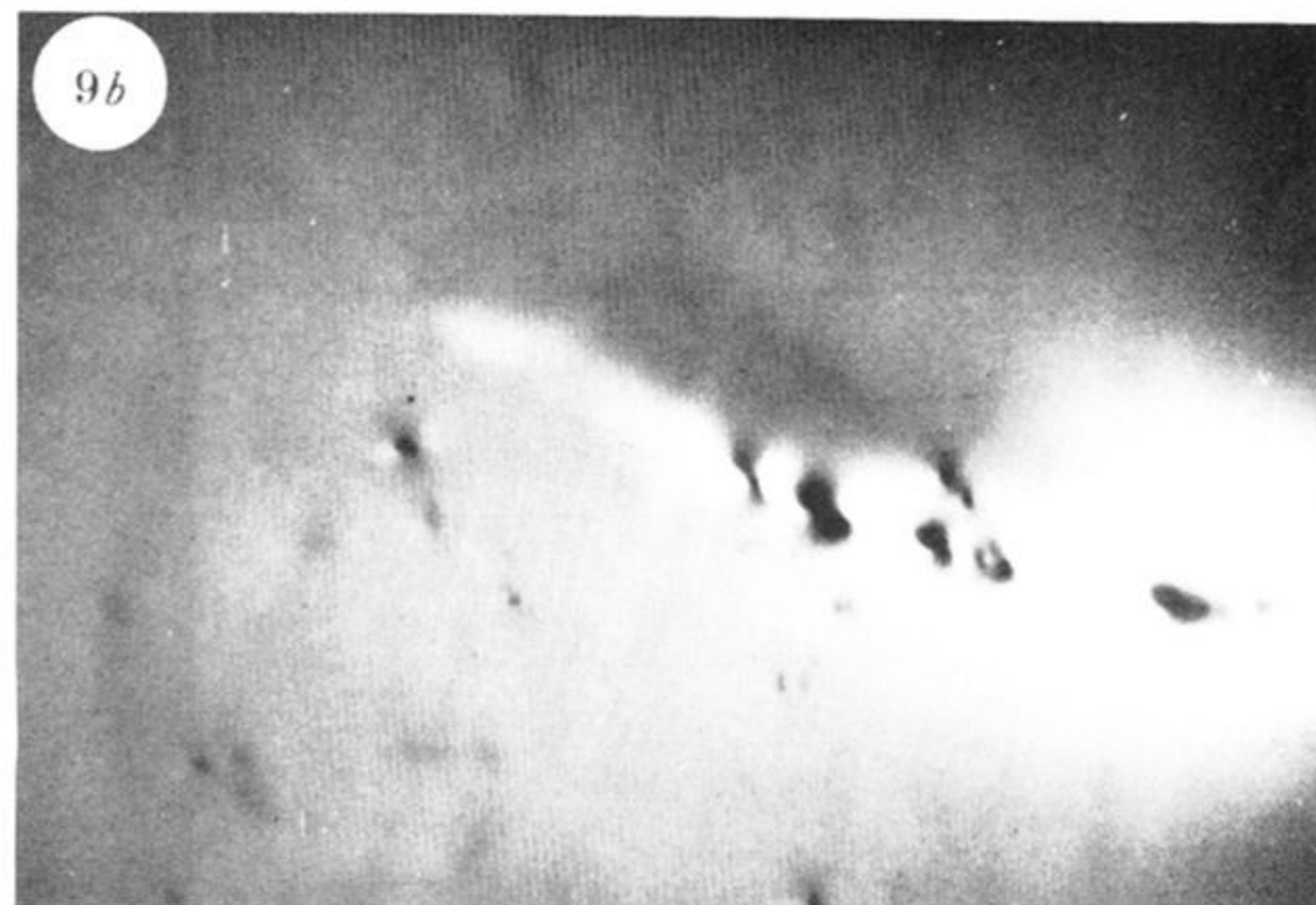
FIGURE 9. (a) SE image of a crack in polystyrene and (b) SEAM image showing craze extending beyond the crack tip. The specimen was Cu-coated and imaged at 20 keV to avoid degradation.
